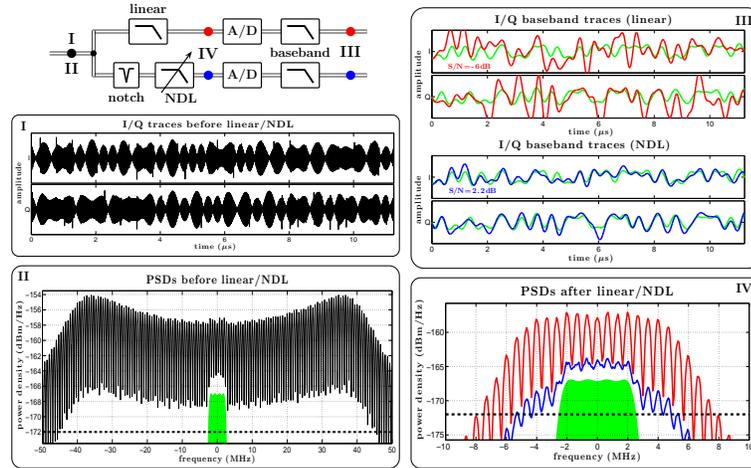
FIGURE 3. Time domain I/Q traces and PSDs of the signals measured at the test points indicated by the fat colored dots on the signal path diagram in the upper left of the figure.
