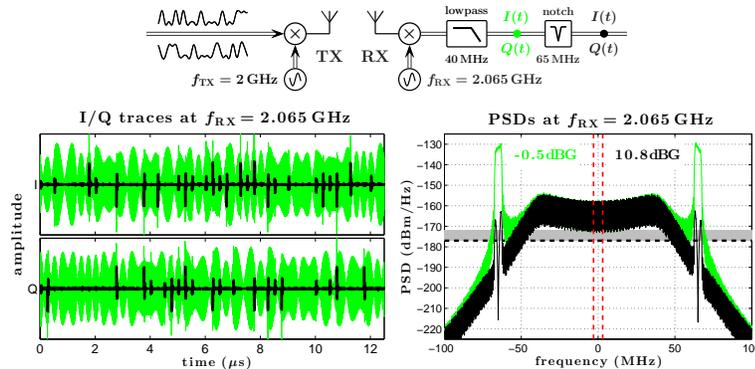
FIGURE 1. In-phase/quadrature ( $I/Q$ ) signal traces (left panel), and PSDs (right panel) for a 40 MHz lowpass filter (green lines), and for a 40 MHz lowpass filter cascaded with a 65 MHz notch filter (black lines). The thermal noise density is indicated by the horizontal dashed line, and the width of the shaded band indicates the receiver noise figure (5 dB).
