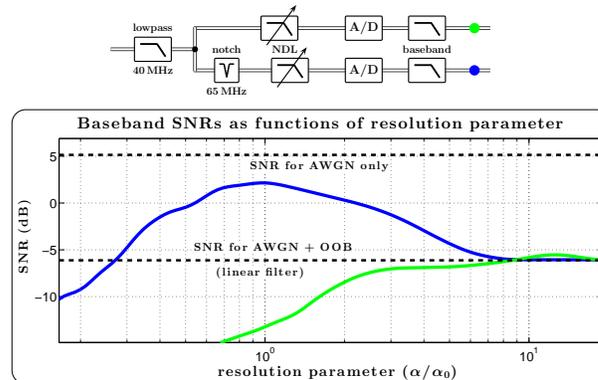
FIGURE 2. SNRs in the receiver baseband as functions of the NDL resolution parameter  $\alpha$  when the NDL is applied directly to the output of the 40 MHz lowpass filter (green line), and when a 65 MHz notch filter precedes the NDL (blue line).
