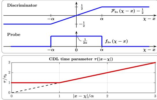
Fig. 2. “Ramp” discriminator and its respective boxcar probe (upper panel), and CDL time parameter  $\tau = \tau(|x - \chi|)$  (lower panel).
