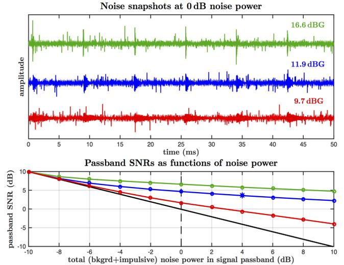
Fig. 4. SNRs as functions of total noise power (lower panel), and snapshots of time-domain input noise traces observed for 0 dB passband SNR (upper panel).
