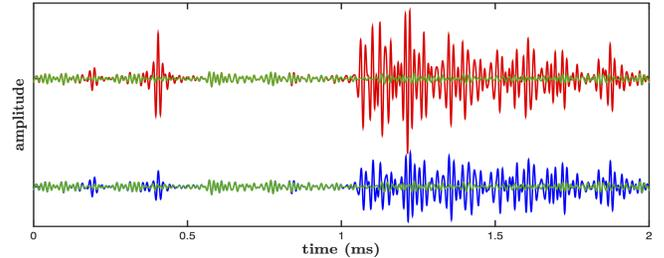
Fig. 5. Example of passband noisy signal traces obtained without (red line) and with NDL (blue line).
