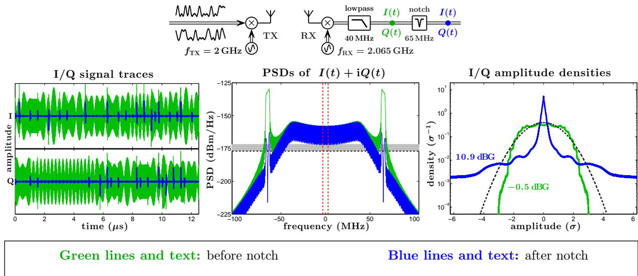
Note that the notch filter reduces the sub-Gaussian part of the interference without affecting the signal of interest and/or the PSD of the impulsive interference around baseband, enabling its effective mitigation by nonlinear filters such as Nonlinear Differential Limiters (NDLs). Linear filters are converted into NDLs by introducing feedback-based nonlinearities into filter responses as illustrated further.
