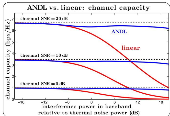
Replacing certain analog filters in the receiver by ANDLs provides resistance to man-made interference
