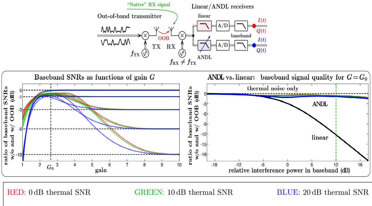
The technogenic out-of-band (OOB) interference affecting the “native” receiver signal is produced by the OOB transmitter, and the baseband signal quality (baseband SNR) is compared for the linear and the ANDL-based receivers for 3 initial (“pre-interference”, or purely thermal) SNRs (0, 10, and 20 dB), and 5 relative OOB interference powers (no interference, and 1, 3, 6, and 10 dB interference relative to the thermal noise power).
