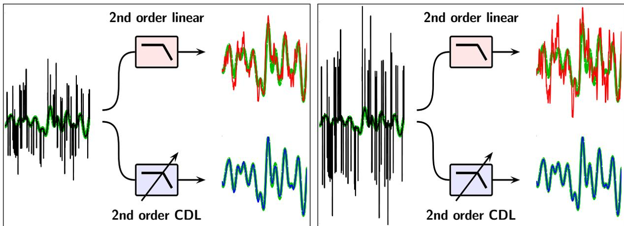
Linear filter: Output noise is proportional to input noise
