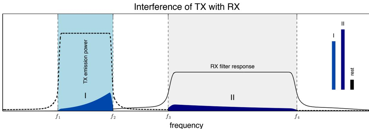
Qualitative illustration of different contributions into the interference which a receiver (RX) experiences from a transmitter (TX)
