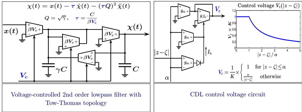
The sub-circuit in the left-hand panel corresponds to the  $\kappa$ -controlled lowpass filter shown in the figure on page 4, and the sub-circuit in the right-hand panel corresponds to the control signal circuit (CSC) shown in the figure on page 4.
