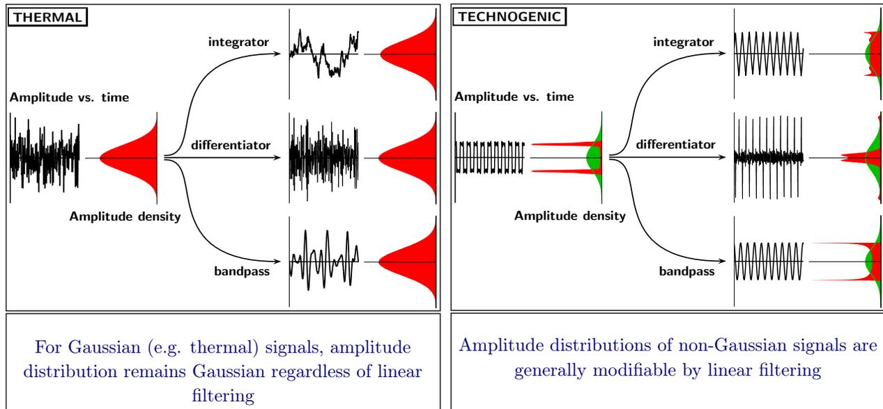
At any given frequency, linear filters affect the power of both the noise and the signal of interest proportionally, and cannot improve the SNR in passband. Nonlinear filters, however, can reduce the PSD of non-Gaussian interference in passband without significantly affecting signals of interest, and thus can increase the passband SNR and the channel capacity.
