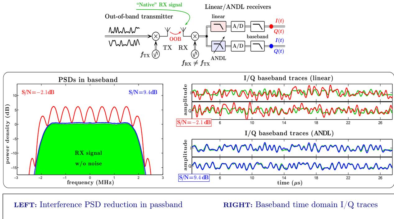
The left panel shows that ANDLs can reduce the spectral density of a man-made interference in the signal passband without affecting the signal of interest. This can be deduced and gauged from observing how the quasiperiodic structure of the PSD is affected by the ANDL in comparison with the linear filter. As a result, the baseband signal quality is improved.
