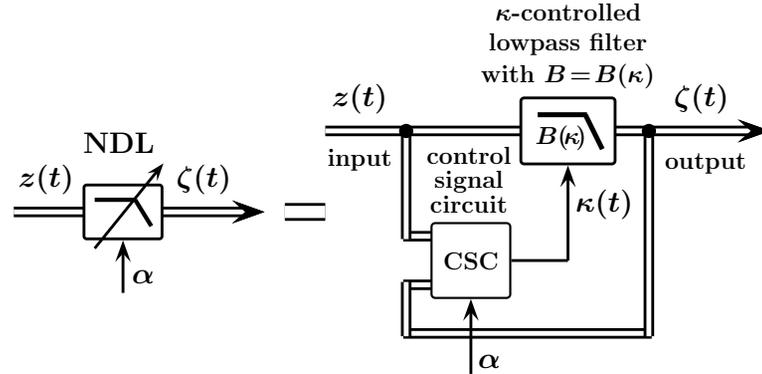
Block diagram of Nonlinear Differential Limiter
